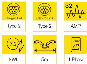
• Suitable with all fully electric & plug in hybrid vehicles
